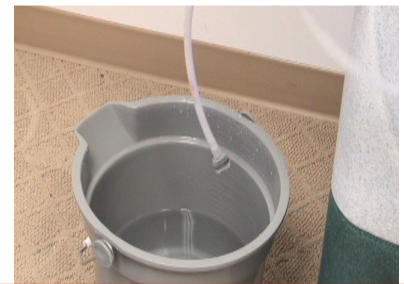
Place Chemical Feed Hose into Rinse Solution
